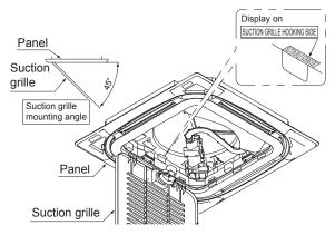
(2) As shown in the illustration, hook the fall prevention cords for the suction grille to the corner clasps (on two corners).
