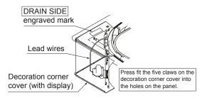
(3) Hook each of the cords of the remaining decoration corner covers (i.e., three covers) onto the corresponding pin on the panel.
