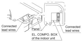
(6) Guide the lead wires through the hook.
