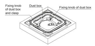
(1) Turn the two fixing knobs of the dust box.
