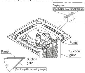
(2) As shown in the illustration, hook the fall prevention cords for the suction grille to the corner clasps (on two corners).
