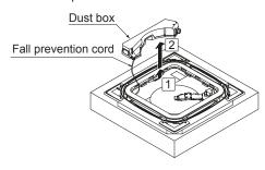
(3) Remove the fall prevention cord for the dust box from the clasp bracket of the panel.
