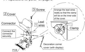
(2) Attach the decoration corner cover (with the display) to the corner with the DRAIN SIDE engraved mark. Push the connected lead wires through the corner hole onto the backside of the ceiling.
