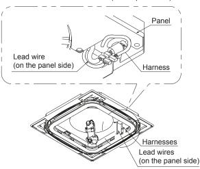
(3) Connect the connectors of the lead wires and move the glass tube to cover the connector part.
