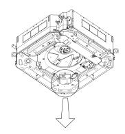
(1) Remove the bypass hole closing cap.
