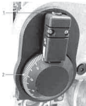
Fig. 7-5 Setting the air throttle
